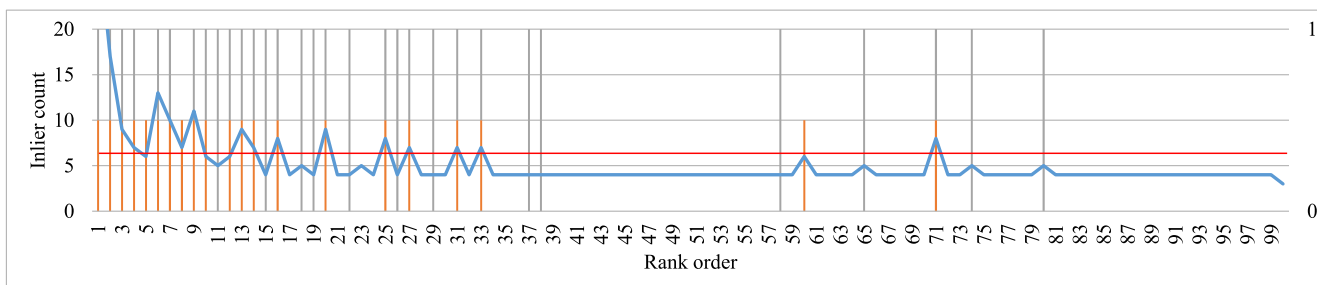
Fig. 6 The blue line shows the total number of inliers found in the top 100 images of the initial rank on the sample query with a baseline AP of 30.14%. The gray bar shows the true positive images appearing in the ranked list, whereas the orange bar shows images selected by our adaptive inlier threshold (ADINT) seen in a red line that yielded a final AP of 82.07%.
