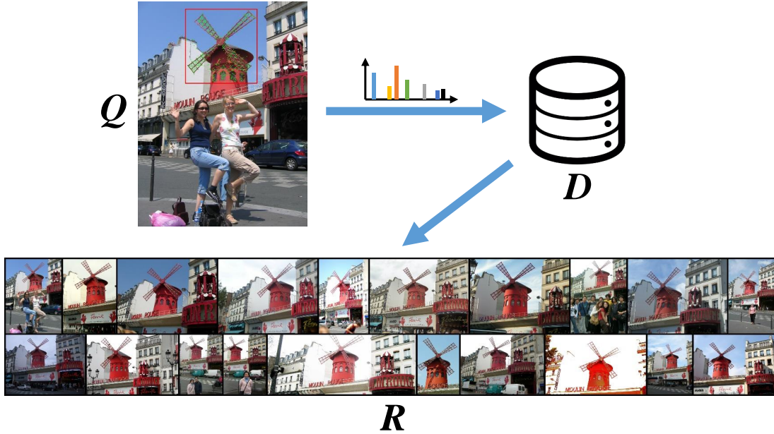
FIGURE 1.10: An example of object-based image retrieval using ROI as a specified object on top of a query image Q . Retrieval is done on an inverted index database D . A rank list R is a similarity result ordered by a score between Q and each of matched image in D .
